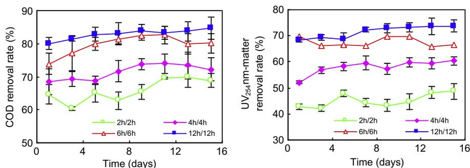
Fig. 1. The removal efficiencies of COD and UV<sub>254</sub> nm-matter in different running modes.
