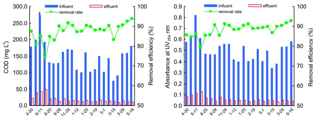
**Fig. 3.** The influent and effluent concentrations and the removal efficiencies of COD and UV<sub>254</sub> nm-matter treated by the multi-level bioreactor from April 2007 to May 2008. The influent and effluent were sampled from B1 and B6 sampling sites, respectively.
