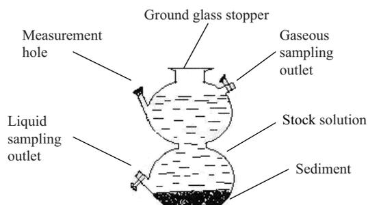
Fig. 2 Schematic diagram of the self-made airtight reaction system.
